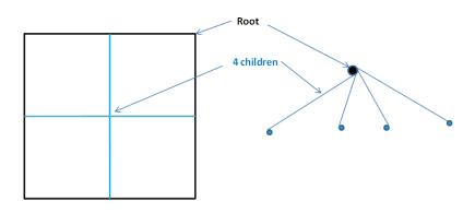
Figure 2 a quad and its corresponding representation
