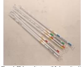
Figure 1: High security straws (0.3ml capacity with weighted ID rod 30mm)
